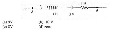
Q 9. AB is a part of circuit. Find the potential difference  $V_A - V_B$  if (a) current I = 2A and is increasing at the rate of 1 A/s (b) current I = 2A and is decreasing at the rate of 1 A/s
